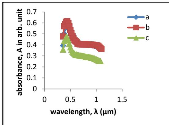
Figure 2: The absorbance versus wavelength of the  $\text{Ag}_2\text{Se}$  thin films deposited at different volume concentrations of TEA. (a) 5ml, (b) 10ml, and (c) 15ml
