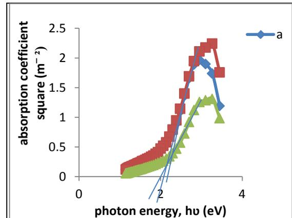
Figure 4: Plot of  $\alpha^2$  versus  $h\nu$  of the  $\text{Ag}_2\text{Se}$  thin films deposited at different concentrations of TEA (a) 5ml, (b) 10ml, and (c) 15ml.
