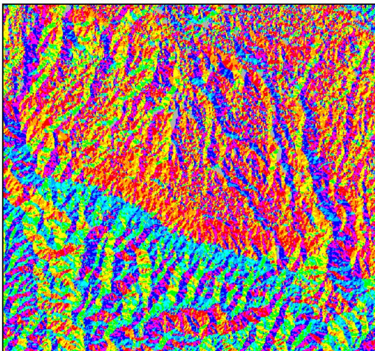
Figure 8: Aspect Map for the Part of the Study Area in Figure 6 Generated from the DEM
