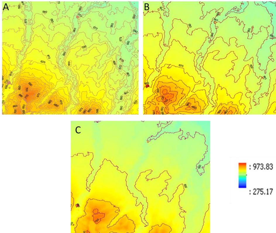
Figure 5: Contour Maps for the Study Area at 10 m (A), 20 m (B) and 50 m (C) Contour Intervals
