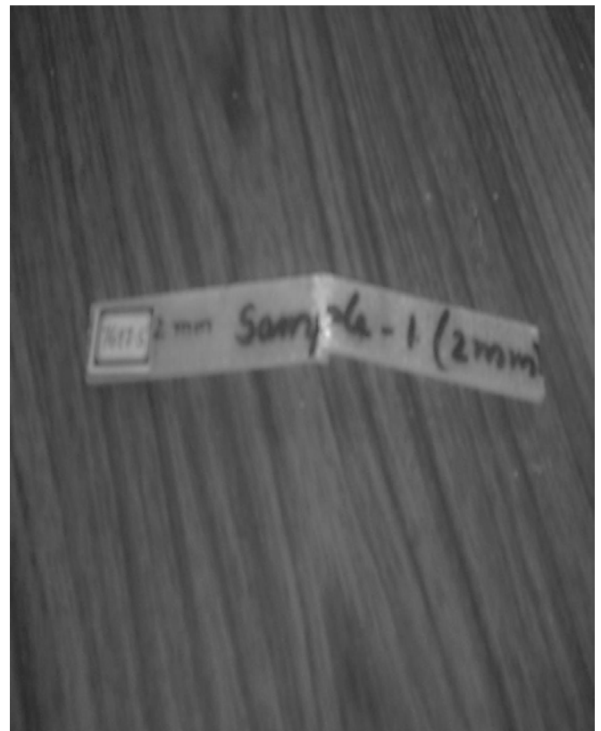
Fig – 3 Sample Specimen Damaged due to Bending
