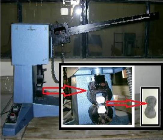
**Figure 2: Tensile Test Machine**
