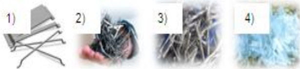
Fig. 5. Geometrical characteristics of the fibers used in our study: 1) Metallic Fibers RC80/50. 2) Metallic Fibers ESF 25. 3) Macro-synthetic Fibers. 4) Micro-synthetic Fibers.
