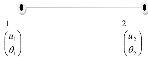
Figure 2: Degrees of freedom on a beam element
