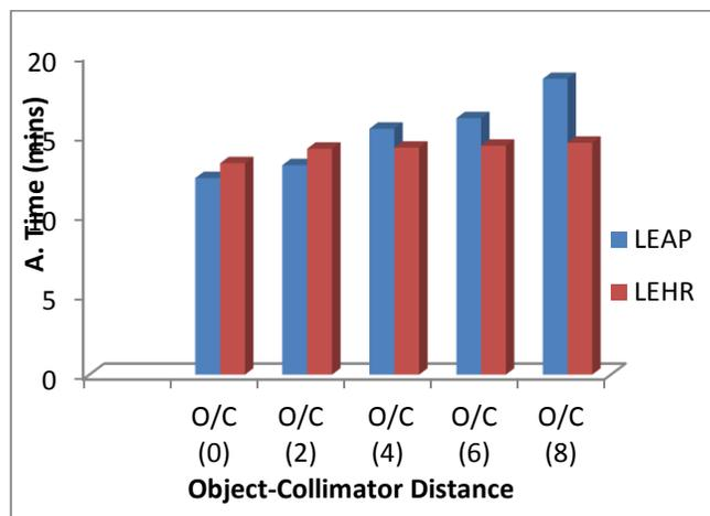
**Figure 3: a graphical relationship between LEAP and LEHR collimators and Acquisition Time with varied object-collimator distance and Acquisition Time (A. Time).**
