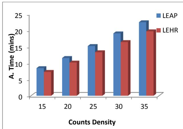
**Figure 2: a graphical relationship between LEAP and LEHR collimators and Acquisition Time with varied count density.**
