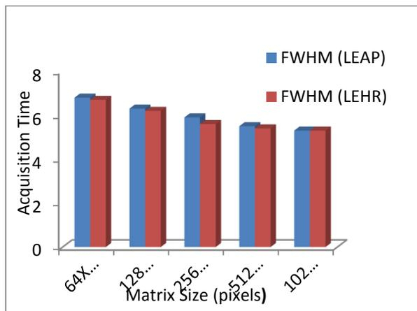
**Figure 1: a graphical relationship between LEAP and LEHR collimators and Acquisition Time with varied matrix size.**
