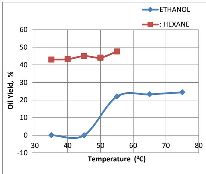
Figure 1: Oil Yield obtained during Neem Oil Extraction at different Temperature using Ethanol and Hexane
