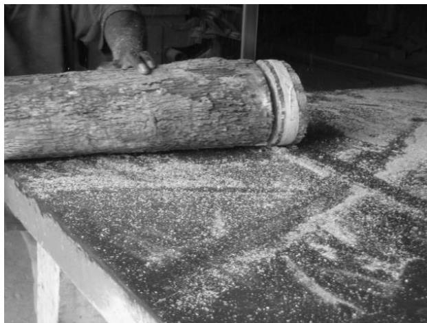
Figure 3: Picture showing the sawn of 5 cm thick disc.
