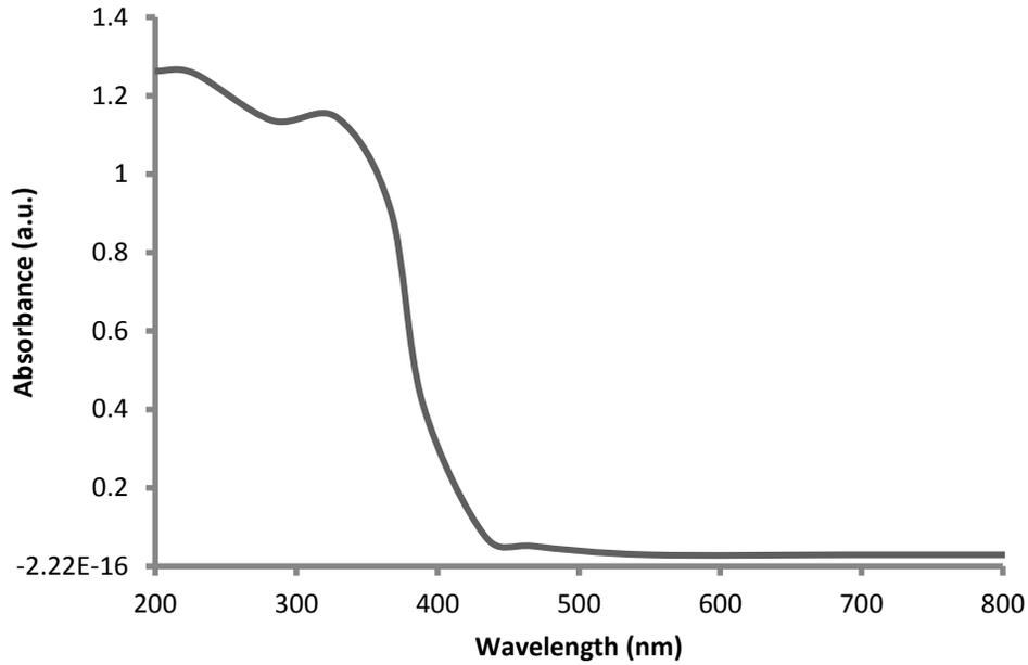
Figure 1. UV-vis spectra of nanoporous titanium dioxide<sup>8</sup>
