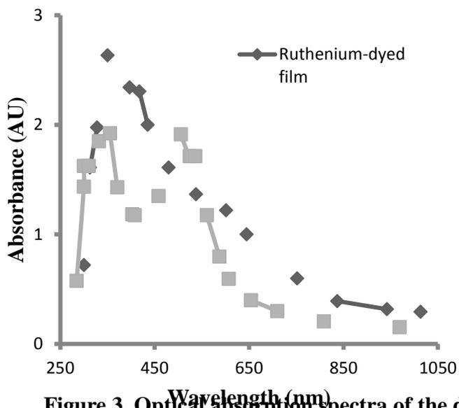
**Figure 3. Optical absorption spectra of the dyed nc-TiO<sub>2</sub> films**
