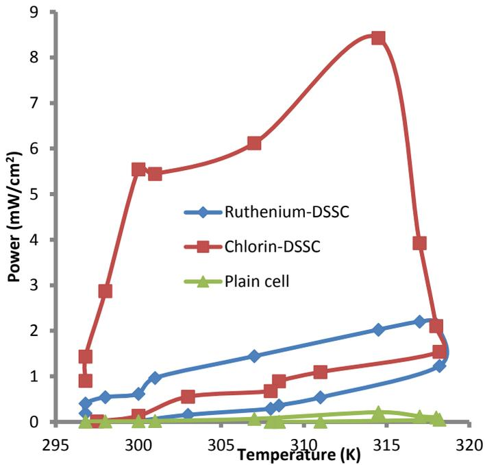
**Figure 5. Power-Temperature curves for the cells (Day 1)**
