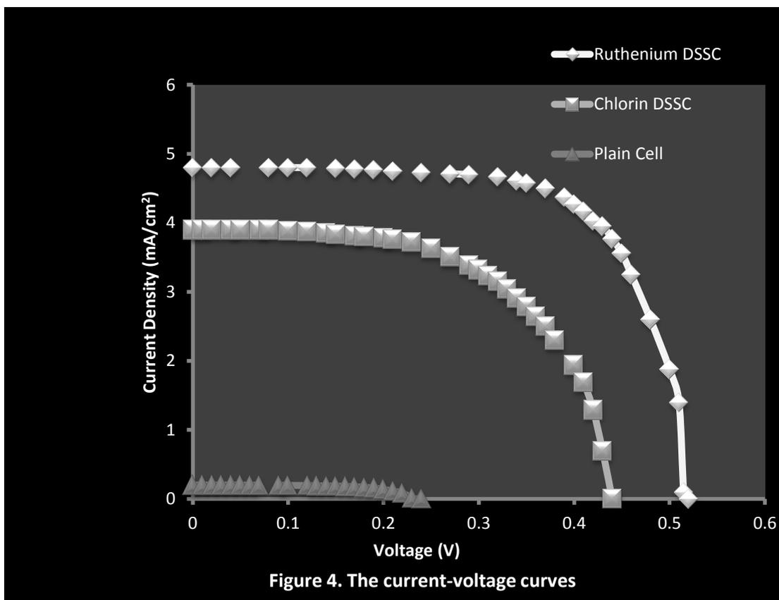
**Figure 4. The current-voltage curves**
