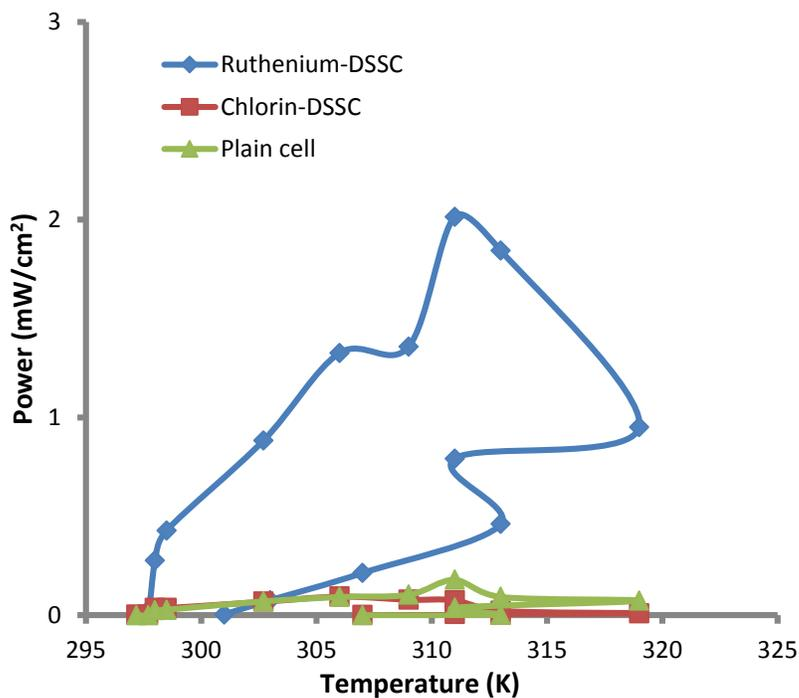
Figure 7. Power-Temperature curves for the cells (Day 3)
