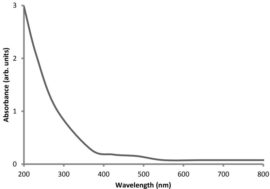
Figure 2. Optical absorption spectra of a finite segment of titanium dioxide nanowire<sup>18</sup>
