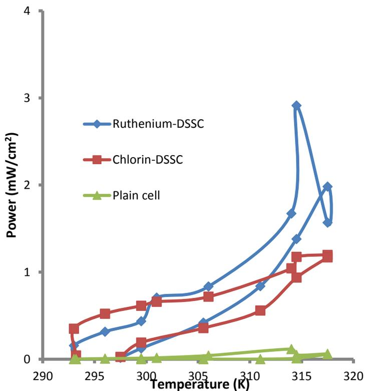
Figure 6. Power-Temperature curves for the cells (Day 2)
